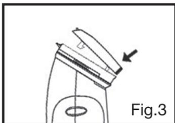
Step 3 Line up rear tab with opening in lower blade.
