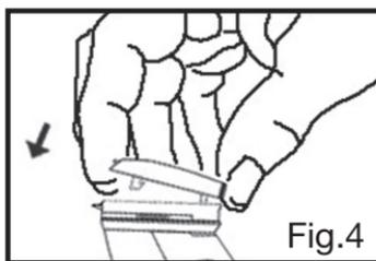
Step 4 Insert the rear tab, slide forward until the 2 front tabs drop in and the blade snaps in place.
